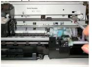
When the print head contacts paper: Move the chassis rail towards the marks. When print quality deteriorates: Move the chassis rail towards the marks.
